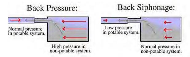
Outside water taps and garden hoses tend to be the most common sources of cross connection contamination at home. The garden hose creates a hazard when submerged in a swimming pool or when attached to a chemical sprayer for weed control. Garden hoses that are left lying on the ground may be contaminated by fertilizers, cesspools, or garden chemicals.
